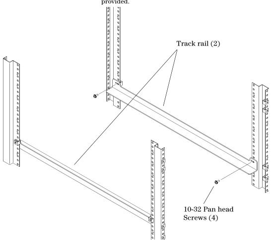
*3* Install track rails to rack using the 4 10-32 pan head screws provided.
