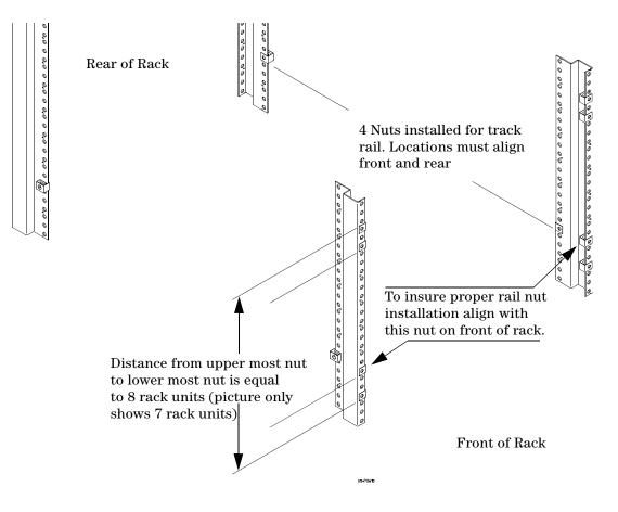
2 The above graphic indicates proper locations for sheet metal nut locations. Note to insure a level installation, the same 8 rack unit locations are used on each vertical rack piece. NOTE: The picture only shows 7 rack units.
