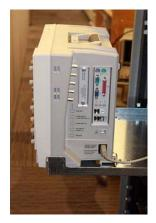
9 Next, push the oscilloscope / support tray into the rack so it is no longer extended. Then connect the other end of each of the cables you routed under the oscilloscope to one of the BNC connectors in the bottom trim plate piece as shown below. If you do not want to install all five BNC connectors into the openings in the bottom face plate then you can fill the hole(s) with the supplied rubber stoppers.
