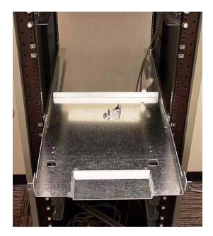
5 Place the oscilloscope on the support tray. There are raised tabs in the support tray. The front side of the oscilloscope's rear feet should rest against these tabs as shown below.
